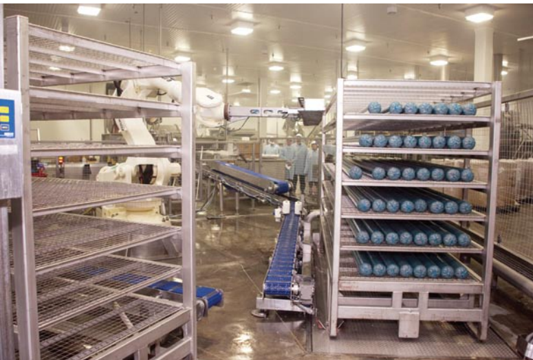
(Left photo) A custom robot arm racks 10-foot-long logs of deli meat, ready to be cooked and sliced. (Right photo) Bags of frozen poultry strips emerge from a form/fill/seal machine on one of two IQF lines in West Liberty Foods' Tremonton plant.
